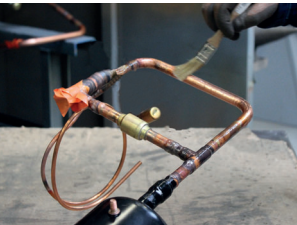
Double varnishing of copper piping and brazing of refrigeration circuit components
